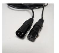
XIR is a common cable, mostly used to connect microphones, speakers and mixing desks.
